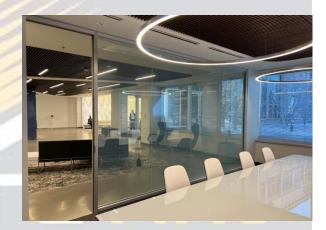
In these 4 pictures of the same conference room, it is easy to see the difference in appearance that PDLC film can have from inside and outside. This is due to different lighting and reflective surfaces. There is also a noticeable difference when looking straight on compared to viewing the glass wall at an angle.
